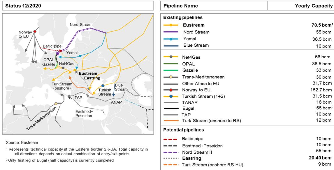
The annual transmission capacity of Eustream's system as of 31 December 2020 was 78.5 bcm in the East-West direction, 55.1 bcm in the North-South direction and 15.7 bcm with respect to the reverse flow (West-East). However, total capacity depends on the actual combination of entry and exit points.
